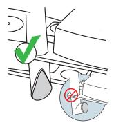
connected to any of the pump inlets. Pop out covers are provided to cover unused inlets. Be sure to cover the unused holes to prevent the pump from collecting debris or insects.
